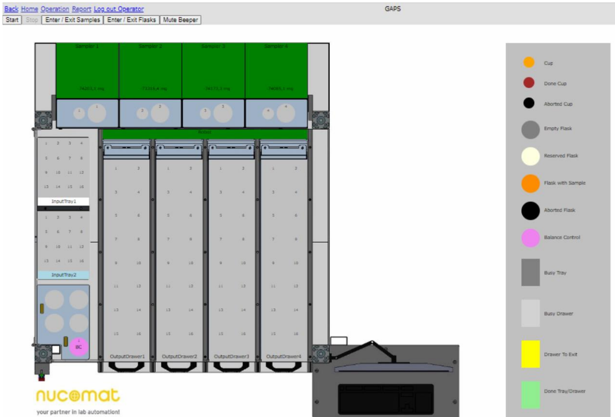
Figure 3: Web interface of the powder dosing system
