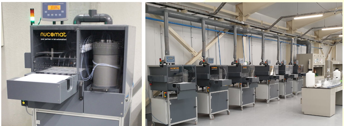
Left: compact dispense; Right: 6 compact acid dispenser units in an analytical lab
